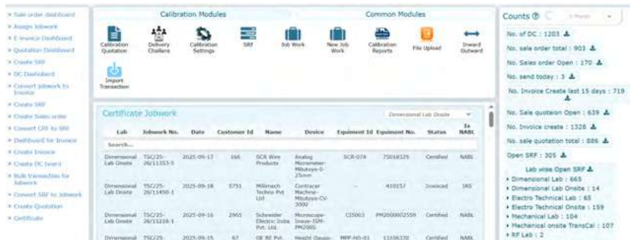
Figure 5. Home dashboard view within the eTransCal system, showing calibration modules, job work listings, and real-time operational metrics.
