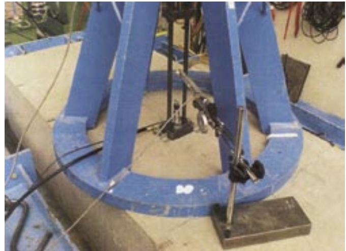
Fig. 4: Test setup for tension test of an anchor
